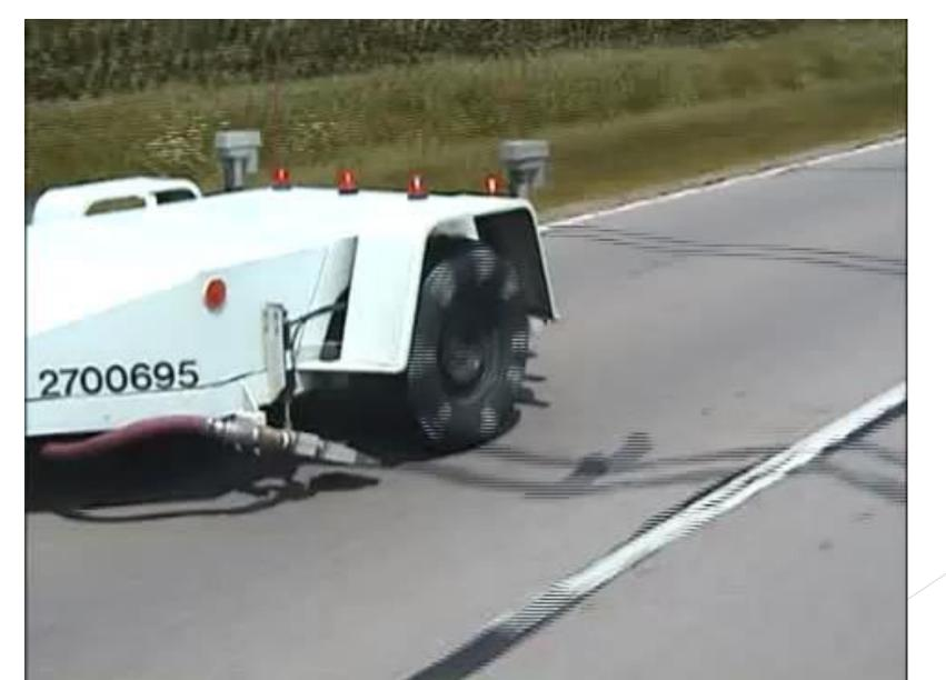
ASTM E 274 Locked Wheel Friction Testing Units
